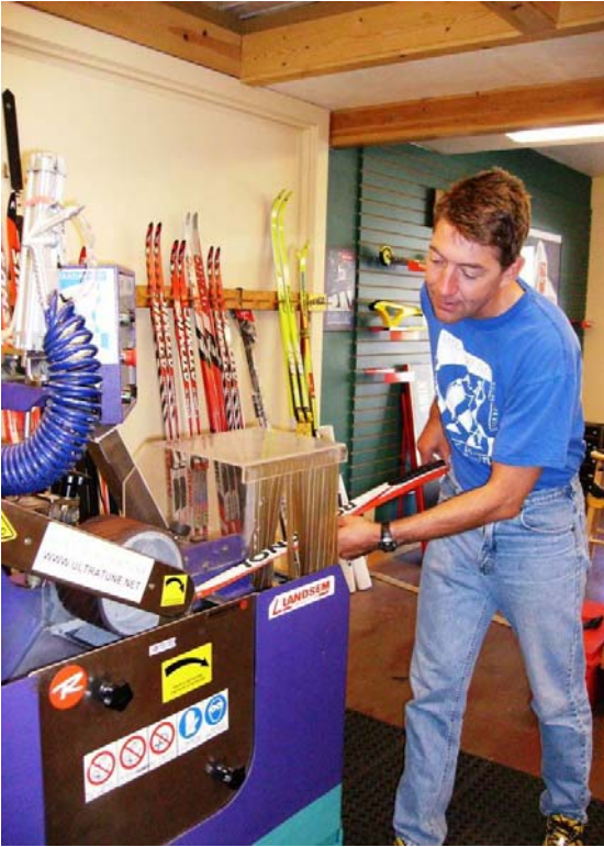
Yes, they can get a grind! Ultratune does careful structuring on the tips and tails of Zero skis and pattern-base waxless classic skis.
